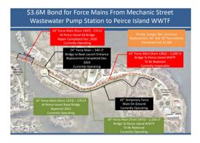
**PEIRCE ISLAND ROAD WORK FOR SEWER FORCE MAINS PROJECT** -- Work continues on the project to replace the force mains to the Peirce Island Wastewater Treatment Facility.
