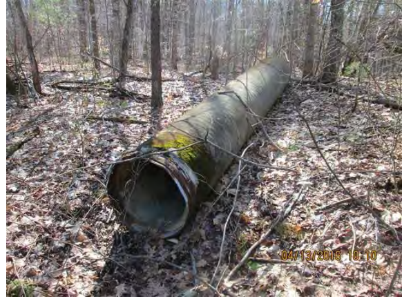
Figure 2-28: 24" PCCP pipe found in woods
