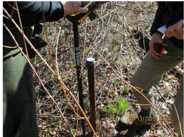
Figure 2-30: Pipe marker found along route
